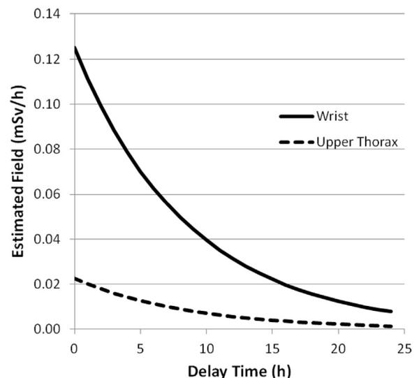
**Figure 4** Radioactive decay. A delay of three or four half-lives is necessary to reduce fields from radioactive source by an order of magnitude. A delay of 24 hours reduces the estimated radiation field by 94%, whereas a delay of only 1 or 2 hours reduces the field by about 10% or 20%. These conservative estimates account for physical decay, not biological elimination, and are based on the model for occupational exposure from right-handed TTE per patient.
